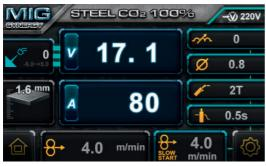
Then use the Left knob (1) to adjust the welding voltage -5~+5V from the standard synergic setting. This will not change the wire speed. It is recommended for ease of use that the wirefeed target speed is adjusted first and then the voltage setting fine- tuned if necessary. Refer to the Welding Settings Quick Reference Chart on page 21 and inside the wirefeed door for recommended common settings.
