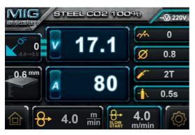
A quick note regarding inductance – this effectively adjusts the intensity of the welding arc. inductance makes the arc 'softer', with less weld spatter. Higher inductance gives a stronger driving arc which can increase penetration. Optimum inductance settings are affected by many welding variables such as: material type, shielding gas joint type, welding amperage, wire size.
